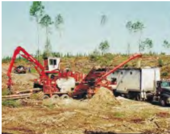
Figure 1. Full-tree logging showing roadside processing.
