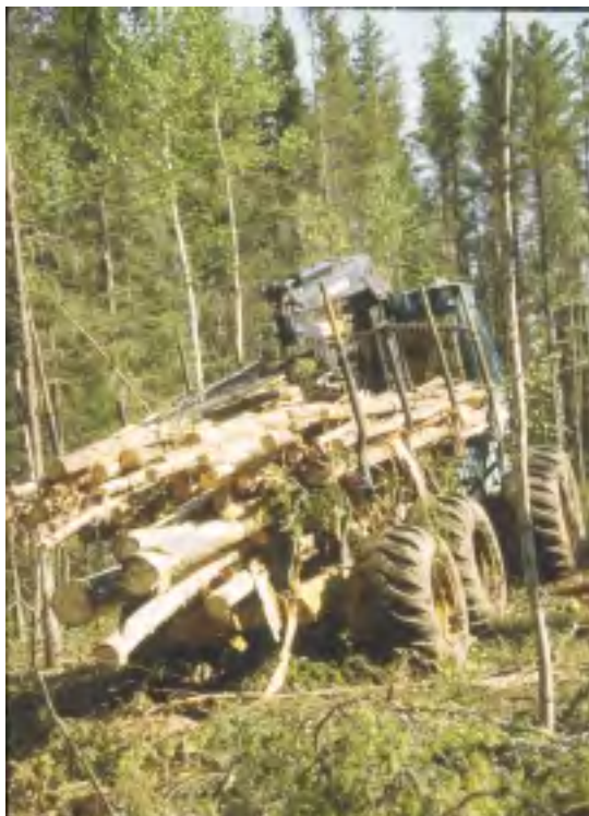
Figure 5. Cut-to-length wood being transported by forwarder.
