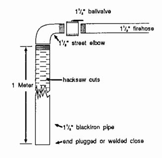
FIGURE 6. Plans for another type of barrel washer.
