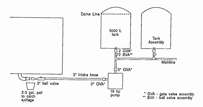
FIGURE 10. Tanker unloading system.
