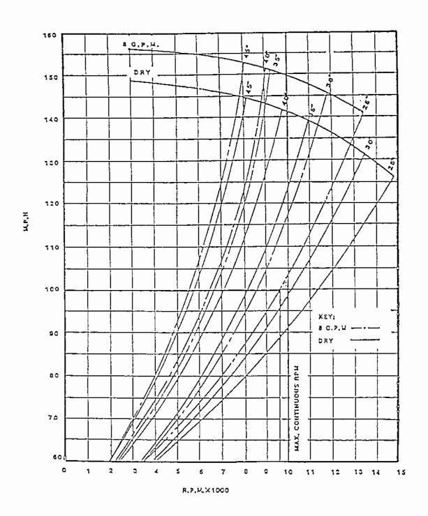
FIGURE 63. Graph of rotational speed vs airspeed-AU4000 13 1/2" twisted blade CBP252-AU4000 5" diameter gauze assembly EX2326/20
