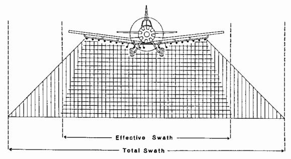
FIGURE 14. Aircraft swath widths.
