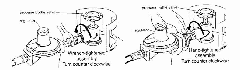
FIGURE 21. Connecting a propane cylinder.
