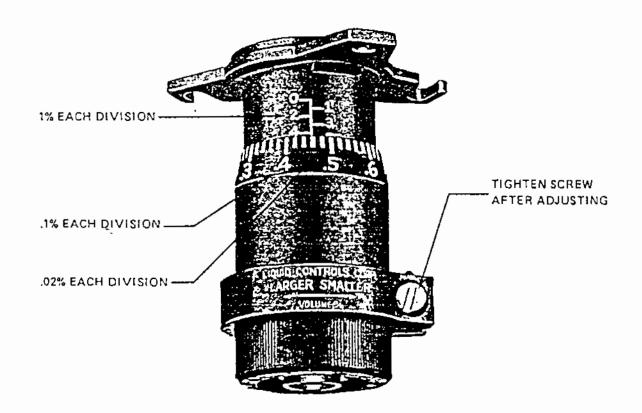
FIGURE 50. Calibration adjuster.
