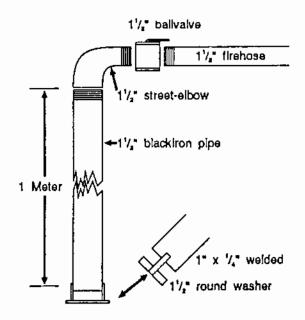
FIGURE 5. Plans for one type of barrel washer.
