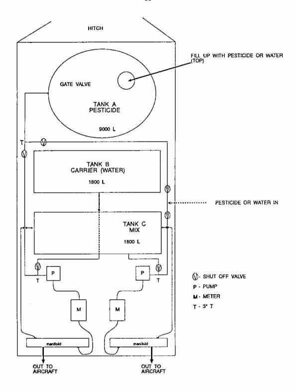
Depending on the mix ratio of carrier to pesticide, storage tanks A and B may change roles from pesticide to carrier storage. For a herbicide mix, the larger tank would togically be used for water, the smaller for herbicide.
