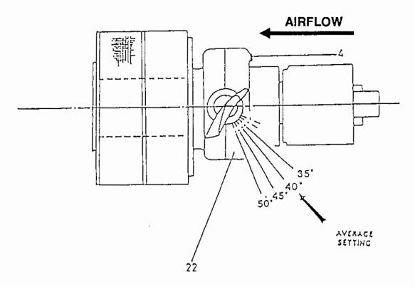
Align pip on blade to appropriate degree line on hub to obtain desired blade angle.
