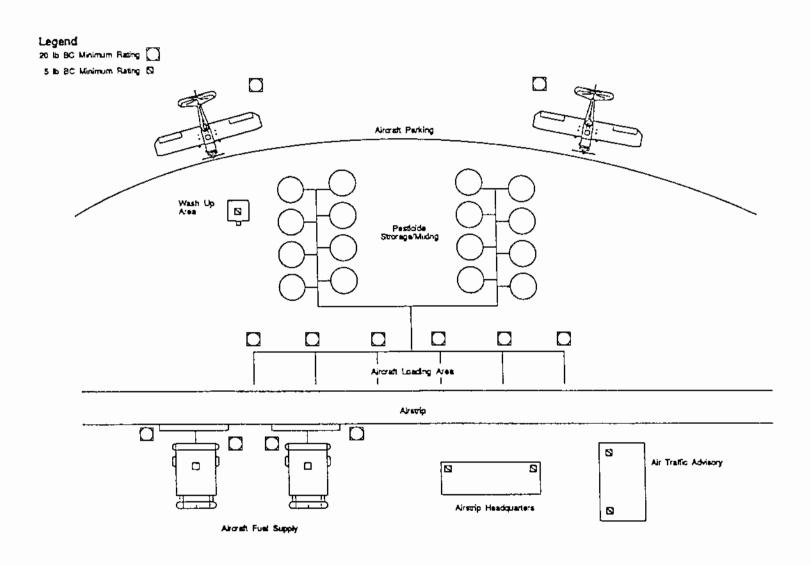
FIGURE 28. Recommended extinguisher placement.
