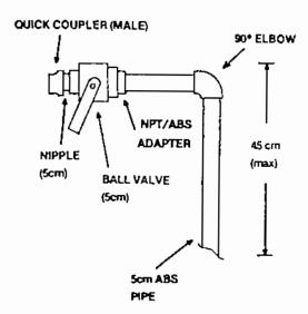
FIGURE 11. Equipment for safe loading of helicopters.
