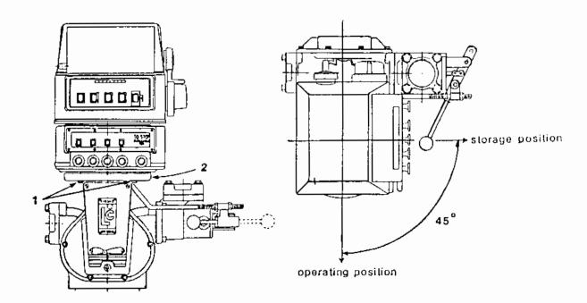
FIGURE 55. Meter head mounting screws.
