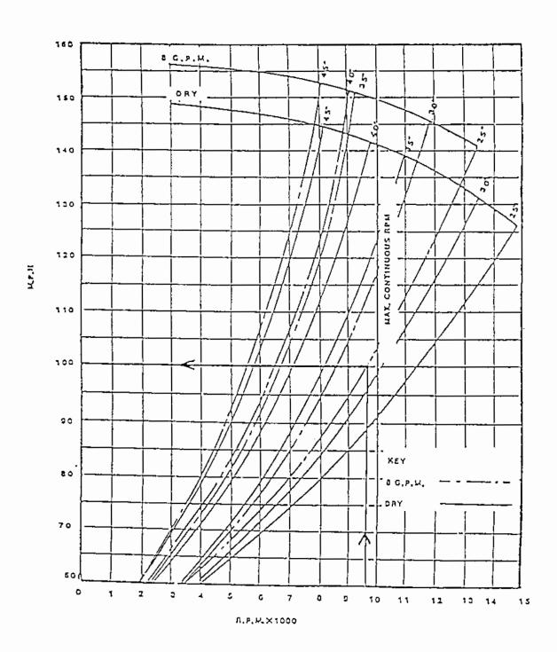
FIGURE 50. Graph of rotational speed vs airspeed-AU3000 13 1/2" twisted blade CBP252-AU3000
