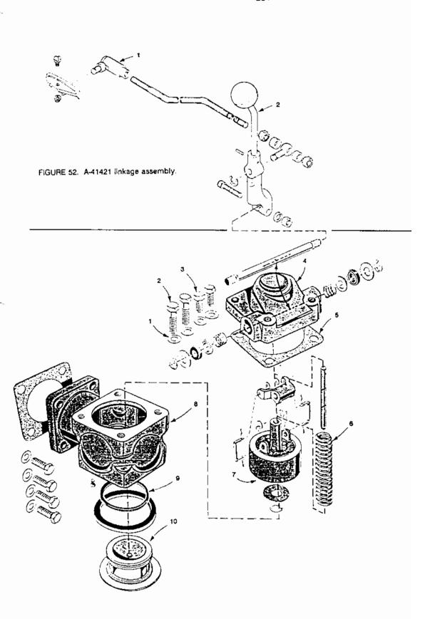
FIGURE 53. A-3620 valve assemblies.
