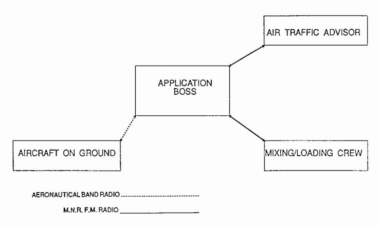
FIGURE 18. Communication links specific to Application Boss.
