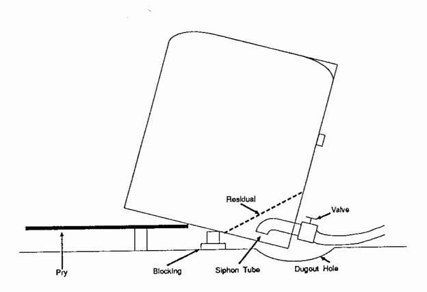
FIGURE 12. Tank draining set-up.
