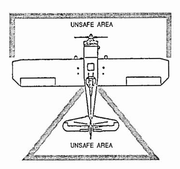
FIGURE 23. Unsafe areas around fixed-wing aircraft.
