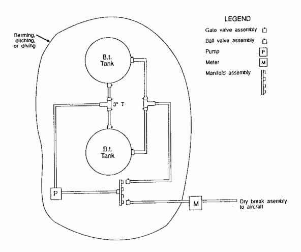
FIGURE 8. Pesticide neat tank farm set-up.
