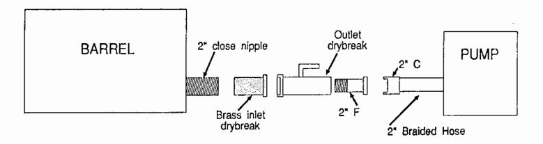
FIGURE 4. Barrel suction method with a drybreak.
