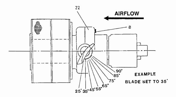
Align appropriate pip on blade with split line of hub to obtain desired blade angle.
