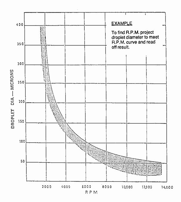
FIGURE 61. Graph of droplet size vs rotational speed for the AU300.
