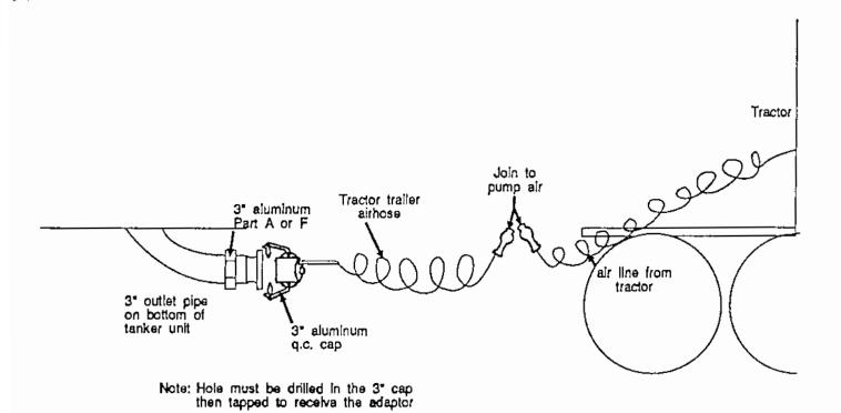
FIGURE 9. Blow back unit attached to tractor.
