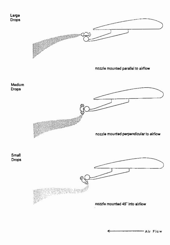
FIGURE 15. Nozzle orientation's affect on droplet size.
