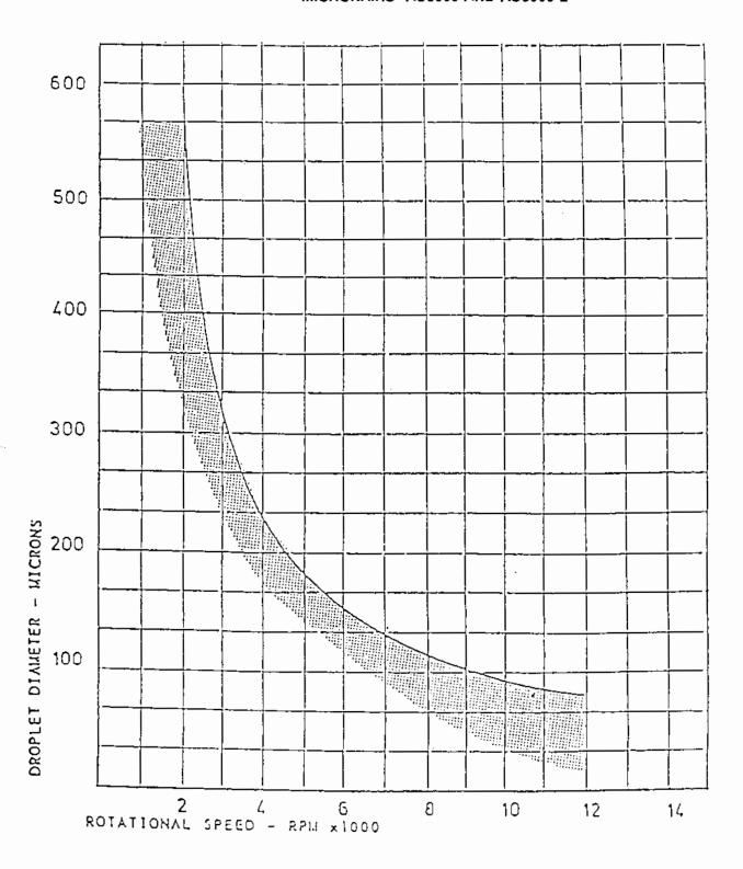
FIGURE 65. Graph of droplet size vs rotational speed for the AU5000 and AU5000-2.
