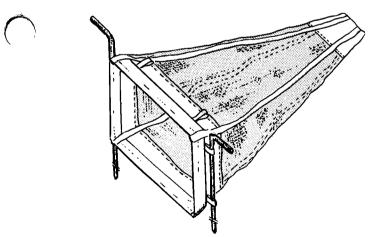
The drift net consists of a rectangular metal or wooden frame on which a nylon net is attached. Two stakes attached to the frame hold the net into the substrate. The net passively collects invertebrates that are carried along in the current (drifting).
