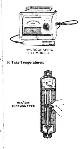
The YSI Telethermometer and the Hydrolab Hydrographic Thermometer are the most common battery operated units in use at this time.
