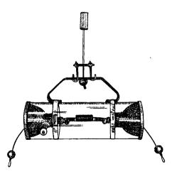
The vertical type Kemmerer bottle, as illustrated, is brass or plastic in construction and is available in different sizes. The most common 1200 model is 6.5 cm in diameter, 64 cm in length and weighs approximately 3 kg.
