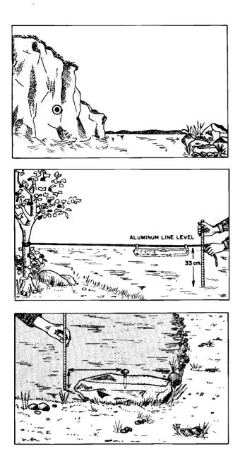
a) Spray paint a circle (not more than 20 cm in diameter) on a flat faced rock, approximately 1 metre above the high water level. Use a star drill to make a hole 2 cm in depth near the centre of the circle.
