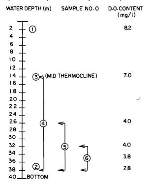
To locate the depth of the 4.0 mg/L dissolved oxygen cut-off proceed as illustrated in the diagram.
