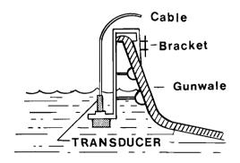
The Transducer must be completely submerged in water to record properly. The face is normally secured to a bracket mounted on the gunwale of the boat. Signals will also penetrate unpainted aluminum and clear ice, as long as the face of the transducer is submerged in water, (alcohol mixture for winter operation). Polyethylene bags are used to hold the liquid in these cases.
