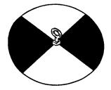
Transparency in lakes is measured with a weighted metal disc, twenty centimetres in diameter with alternate white and black quadrants. This instrument is known as a *secchi disc*. A line, graduated in metres and centimetres is attached to the disc.
