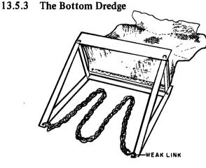
This sampler, or modifications thereof, consists of a heavy metal frame 45 cm x 25 cm to which a 75 cm long nylon net and pull chain (bridle) are attached. A weak link is attached to one terminal of the pull chain to reduce damage to the dredge if it becomes snagged. It is designed to gather aquatic life in deeper sections of the stream (i.e. up to a chest depth).
