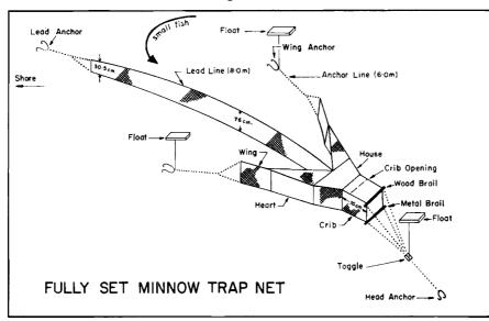
The net is usually set perpendicular to shore with the crib section completely submerged in the deeper water, but not in a water depth exceeding double the net height of five feet (1.5 m).
