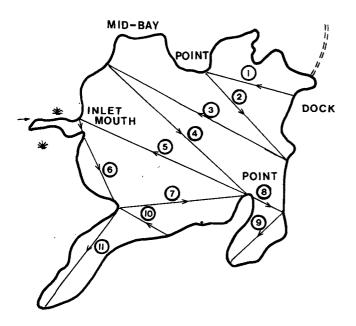
Echo sounding, i.e. running the sounding transect lines is a flexible and schematic procedure in collecting the required depth data for the production of a representative Contour Map.
