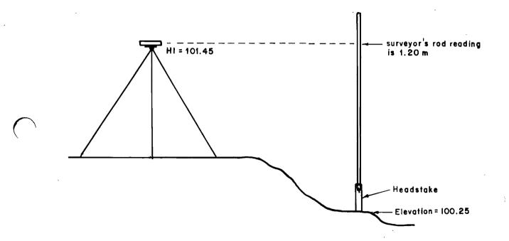
Turning Point (TP): The turning point is a temporary bench mark upon which FS and BS readings are taken to continue a line of levels. This is necessary where a shot may be too long or where there is an obstruction between the instrument and the point to be measured.
