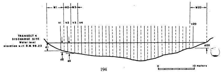
In the preceding diagram of a discharge measuring site, note that the solid vertical lines denote the measuring points for velocity (v) and depth (d). The broken vertical lines denote the limits of the panel width (w). The panels W1 and W20 are both wider than the others to compensate for the edge effect of laminar flow.
