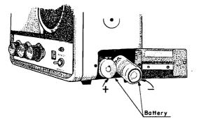
The power supply for both the Furuno and Ferrograph units is a 12V battery (wet or dry cell). Each unit normally has a volt-meter dial to indicate the power supply strength. Furuno models should operate as efficiently with eight *transistor* dry cell batteries as with twelve volt wet cells. You can expect problems though if you use ordinary flashlight batteries.
