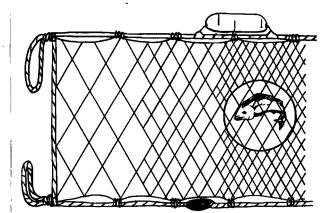
Experimental gangs of either multifilament (nylon) or monofilament nets, are used for sampling larger fish. The recommended minimal gang of nets consists of at least eight different stretched mesh size segments of 1.5 metres in depth and fifteen metres in length. The continuing use of the eight by fifty foot nets in one-half inch intervals is logical and practical, until replacement is required, or until the equivalent metric sized nets are available through suppliers.
