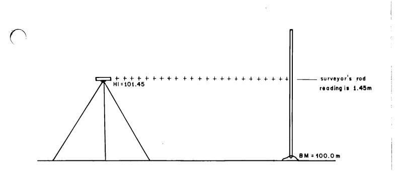
Height of the Instrument (HI): The HI is always the result of a backsight and is the sum of the known elevation and the BS rod reading.
