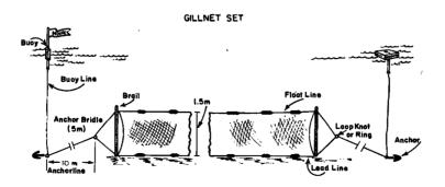
Long anchor lines equalize tensions with the result that there is a compensating effect on the narrowing in of meshes due to site irregularities.
