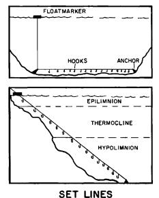
A series of baited hooks (use minnows and small suckers caught by seining) is suspended at desired depth(s). The most common method is the bottom set. A series of hooks (single or treble) is suspended from a stretched line along the basin bottom.
