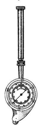
This unit measures linear distance in centimetres or inches. The indicator needle is set at zero by rotating the tracing wheel. Measure the shoreline by tracing the outline of the figure, and then read the result from the scale. Care must be taken so that the indicator needle travels in a positive direction. Also, on a large lake the needle may travel more than once around the circumference of the dial. Therefore, the operator should keep close watch as to the number of revolutions.
