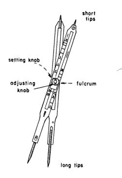
Proportional dividers are instruments made of crossed double pointed metal arms. They are made in such a way (as the name suggests) that they can be adjusted to measure ratios or proportions.
