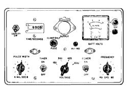
Due to the decreased mortality rate and faster recovery rate of the shocked fish, *pulsed direct current* operation of the unit is recommended. In view of the catchability efficiency of other types of gear in lakes and the high unit price tags, the electrofishing method is presently confined for use in the stream survey.
