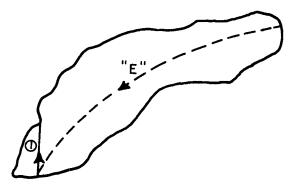
The "E" Line is an exploratory line and will always be the initial line run. If the basin shape is simple (reasonably oval or rectangular without indentations (bays)), then one "E" Line will normally suffice. If the basin shape is more complex, then more than one "E" Line is required. "E" Lines will be run the length of the basin or basin segment, midway between the shorelines. It may not, and it does not need to be a straight line. It will be shown as illustrated on the transect map.
