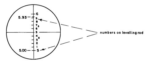
The distance from the level to the rod is determined by reading the rod heights that the stadia cross-hairs have intersected. Subtract the lower reading from the upper reading and multiply by a constant (usually 100, but this may vary with different instruments). For example, upper and lower stadia readings of 5.93 and 5.00 m, respectively, indicate that the rod is positioned 9.30 m (0.93  $\times$  100) from the level.
