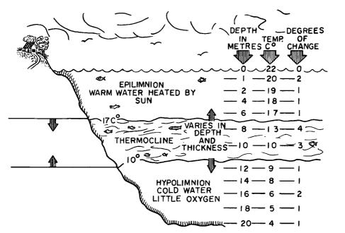
Stratification is the result of the vertical heating of water in a lake basin. A series of vertical temperature records, taken at two metre depth intervals from top to bottom, is illustrated in the diagram above.
